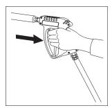
**STEP 3:** Turn garden hose water off. Open the spray gun to relieve remaining pressure.
